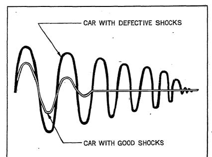
If your car were hooked up to an oscilloscope, measuring the ride, here's the difference a new set of shocks would produce. Comfort, the kind you enjoyed when the car was new, would be restored and there would be less stress placed on vital components like tires.
