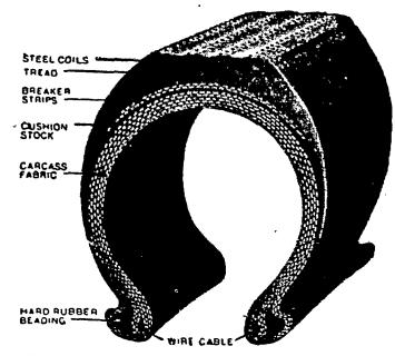
The principle of this tire is made clear by the picture above. Four coils of steel wire, deeply vulcanized into the rubber-encircle each tire After a little use, the outer edges of these coils wearoff, presenting thousands of steel points which, under the load, project and "grip the road like a thousand claws."
