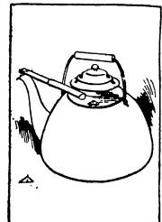
the direction of the spout. This pipe can be extended until the end rests on the tip of the spout, and in this position all the escaping steam is blown straight out from the kettle and cannot float back and burn one. With these two openings air can enter through the
