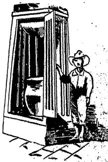
ponderous porous stone, hollowed out to the shape of a wash basin. By a slatwork of saprights it is supported directly over a stone receptacle on the ground. A gallon or two of water in poured into the upper, and falls drop: by drop into the lower. The water is made clear as crystal, and, while the method is slow, it is sure. An inspection of the moss-covered lower half of the upper stone detracts a little from the esteem which the water wins at a first glance.
