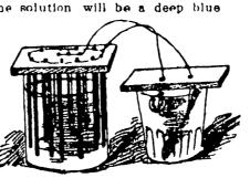
Now provide a large, deep tumbler or a fruit can and into this your the vitriol. Bring over the wire that is connected with the zinc in your battery and to its end tie an old iron key or button hook. Allow this to sink into the vitriol solution. The end of the wire that comes from the copper or carbon of your battery should also be immersed in the liquid. In a few beautifully coated with the copper. It is a process exceedingly interest-
